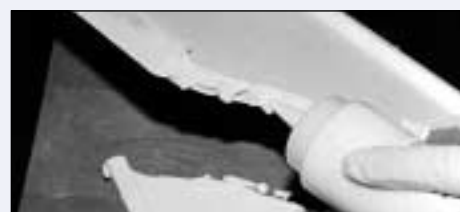
Ceramabond™ 503 repairs mullite sagger.
