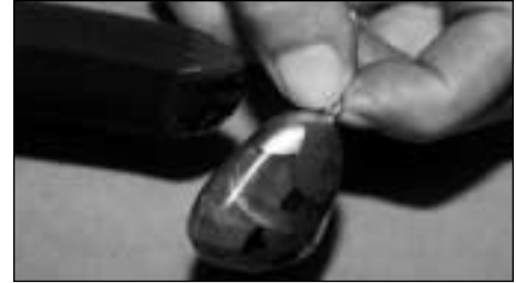
Pyro-Duct™ 598-C metallizes handbag accessory for plating.
